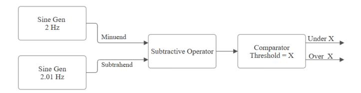
In this diagram you can see the order of processes. It is important to note that the "Under X" and "Over X" outputs from the comparator are gate outputs. This means the output stands "high" or
